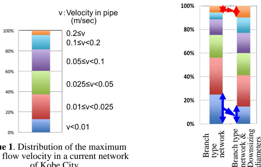
**Figure 1.** Distribution of the maximum daily flow velocity in a current network of Kobe City.
